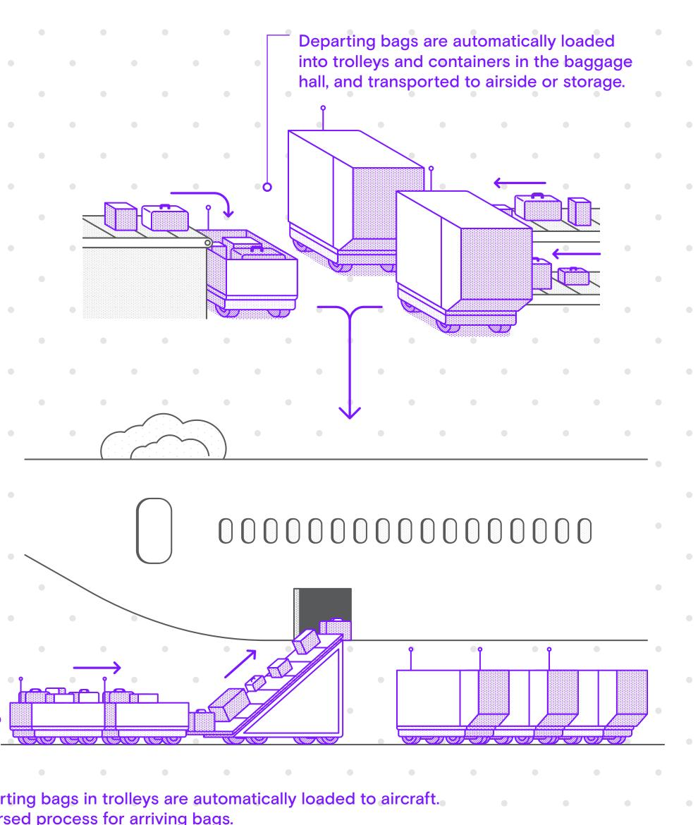
Departing bags in trolleys are automatically loaded to aircraft. Reversed process for arriving bags.
